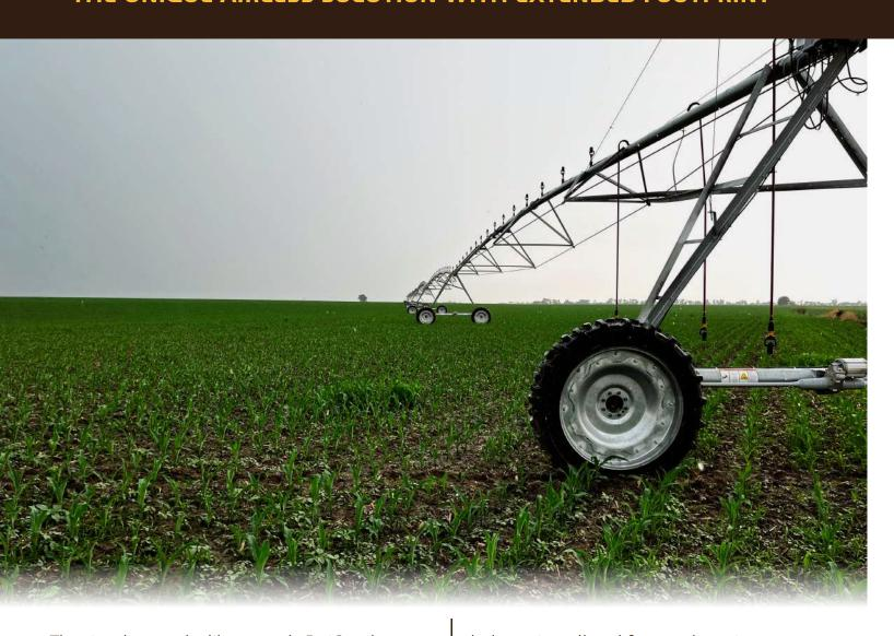
The tire that works like a track: IrriCup by Galileo Wheel - the most advanced innovation in mobile irrigation today. 100% airless tires, no flats. Flexible on drivetrain system, reducing wear and tear. Comes ready to
